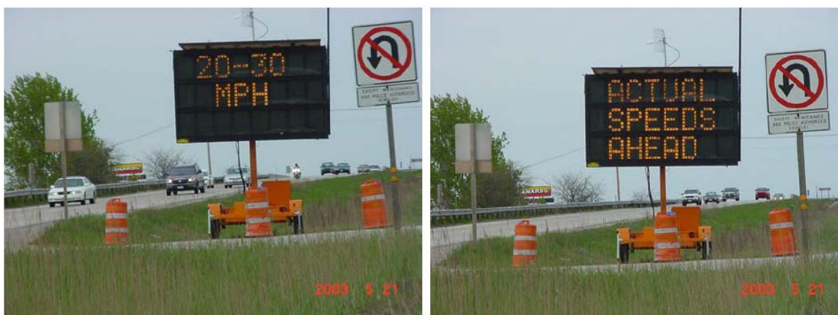
Figure 9. Two Phase Message Display from Intellizone System (55)
